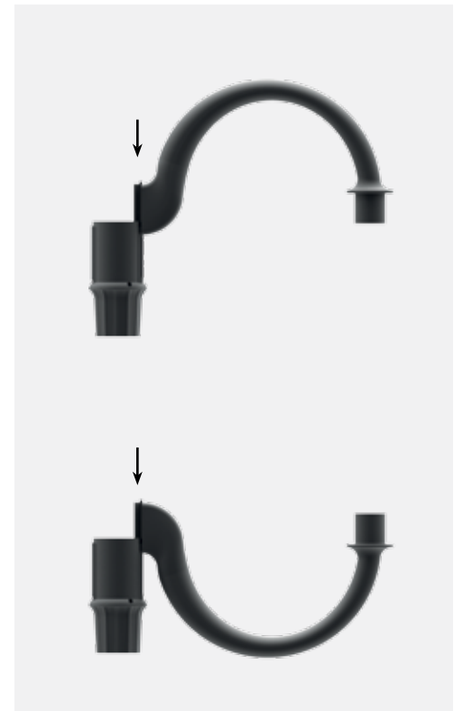
The way of assembling an arm system in head
