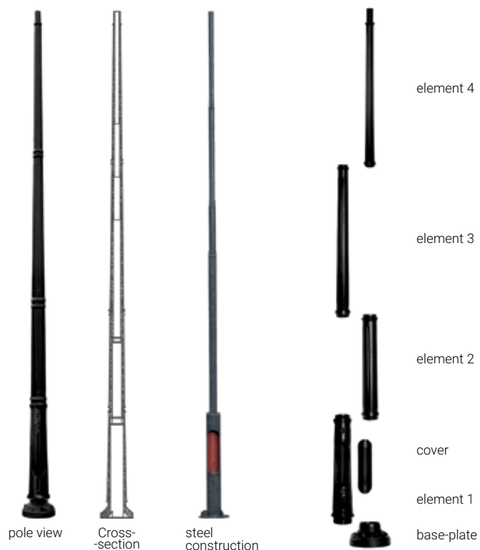
Example of the pole construction SP-4W
